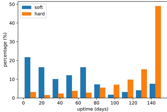
**Figure 9. distribution of uptimes compared on type of probe (hardware/software)**
