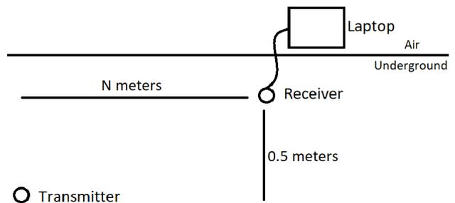
Figure 7. Schematic overview of the first experiment.
