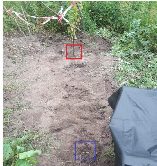
Figure 18. Photo of the set-up for experiment 1. The red box indicates the position of the transmitter, the blue box the position of the receiver. Normally the receiver is buried a bit deeper, but for illustrative purposes that is not the case here.
