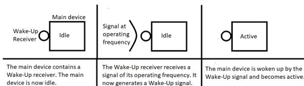
**Figure 1. Schematic overview of Wake-Up mechanics.**
