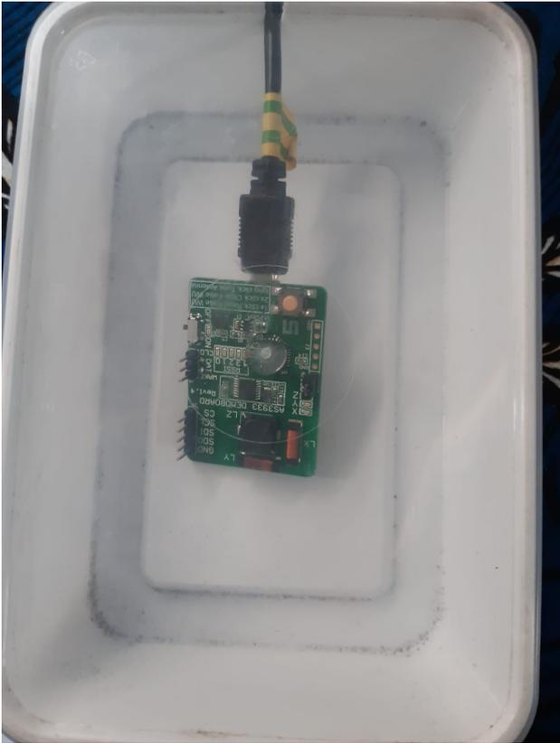
Figure 4. Packaging of the receiver.
