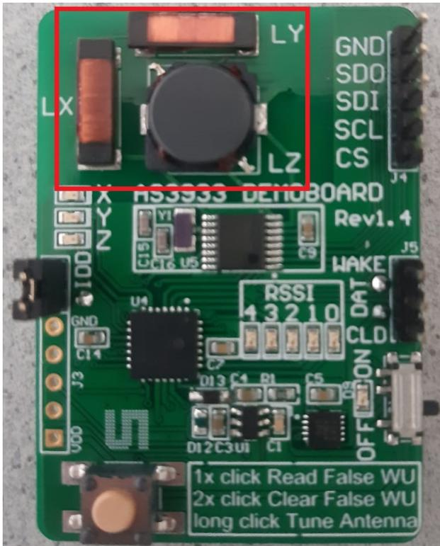
Figure 3. The AS3933 Demoboard.
