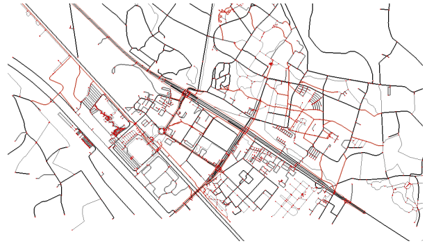
Figure 2. network generated using Netconvert from data of OpenStreetMap of the University of Twente campus
