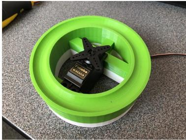
**Figure C.1:** Bottom base and placement of servo motor
