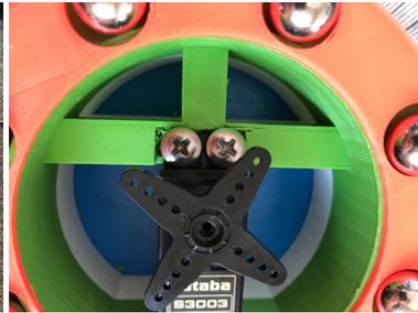
**Figure C.2:** Attachment onto support of bottom servo motor
