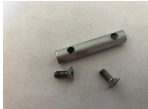
**Figure 4.8:** Connection shaft between screw-thread and motor shaft, where two bolts clamp the shaft to the tube
