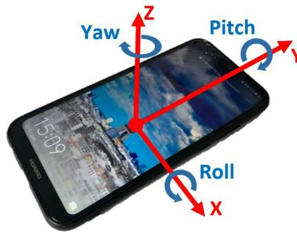
**Figure 3.6:** Definition of frame around mobile phone
