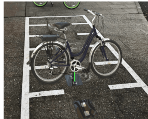
Figure 21. Rx placement on kickstand
