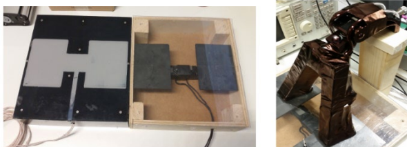
Figure 19. Primary and secondary IPT coils [37]
