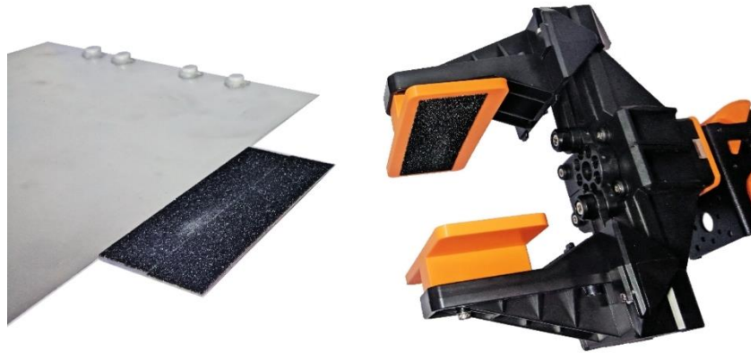
Figure 2: Custom build plate and robotic arm modifications
