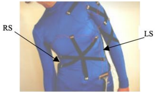
Figure 11: Carbon loaded rubbers strain sensor
