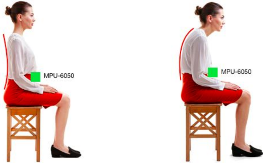
Figure 42: Belly placed accelerometer to measure posture [67]
