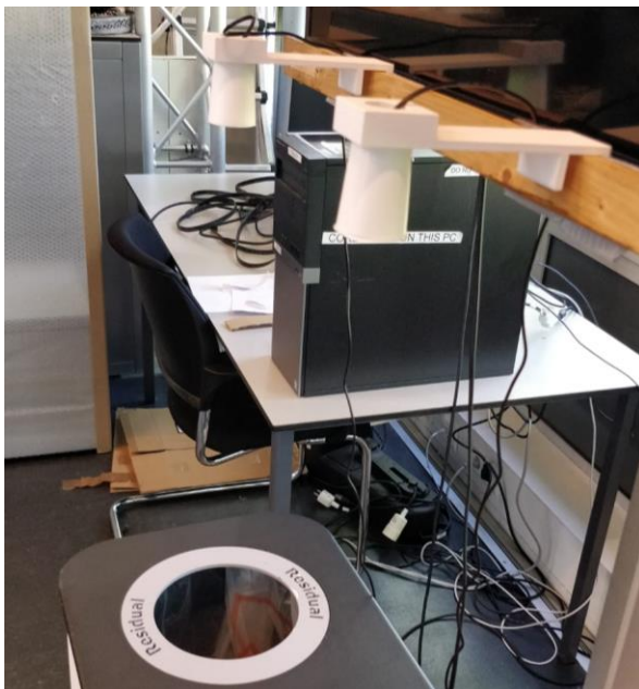
Figure 34: Picture showing ultrasound sensors used in prototype
