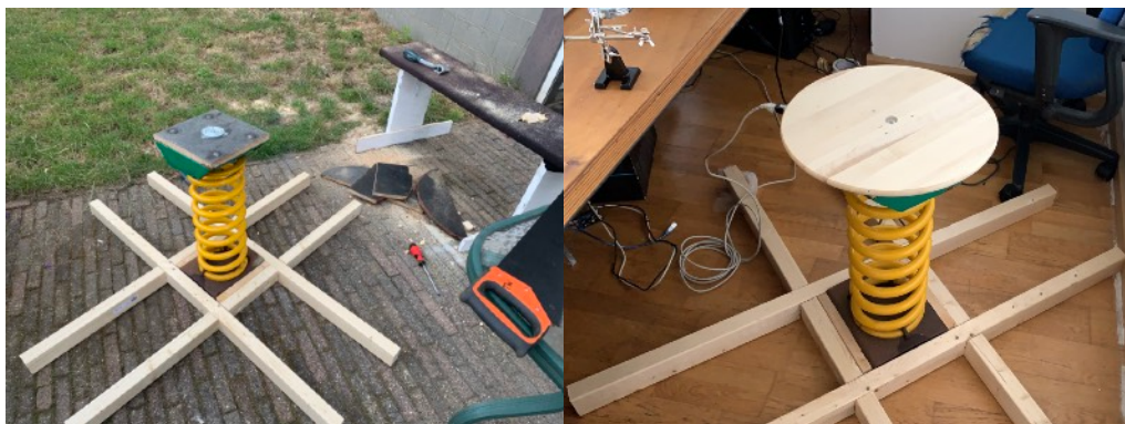
Figure 24: Prototype spring chair
