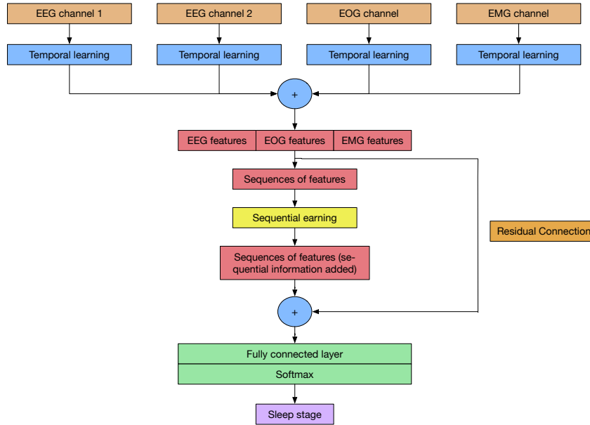
Figure 3.4: Testing model architecture for evaluating the module — adding the residual connection to final feature representations.
