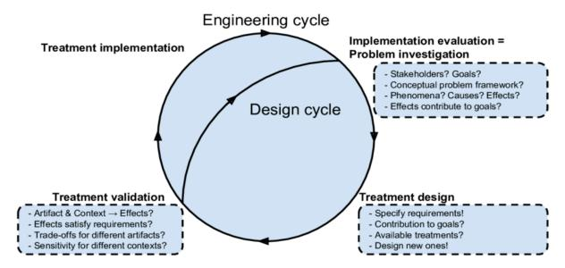
Figure 1.1: The Engineering and Design Cycles
