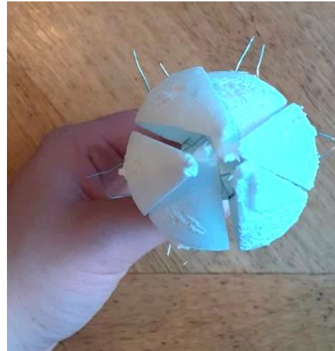
Figure 41 Putting the 3D printed components together using wire and a needle to enlarge the holes
