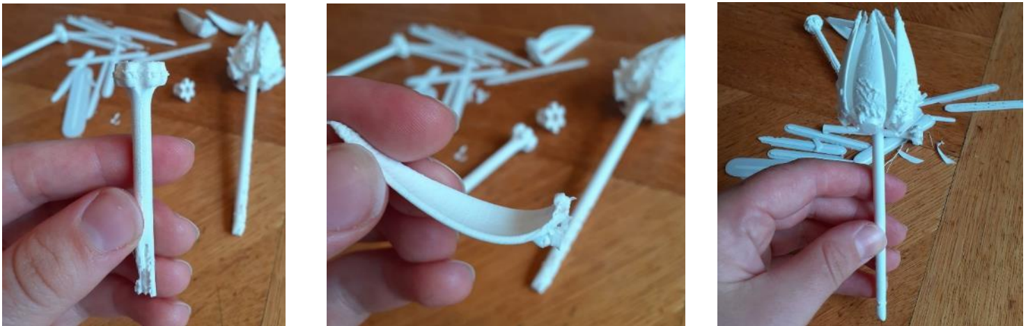
Figure 39 Too small 3D printed parts (three images above)
