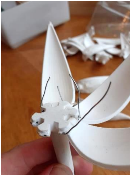
Figure 41 Putting the 3D printed components together using wire and a needle to enlarge the holes
