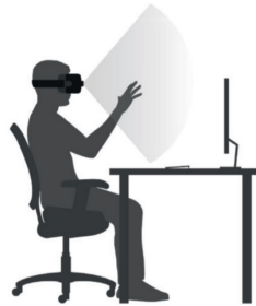
Figure 42: Range of the Leap Motion Controller when placing the controller on a VR headset [63]
