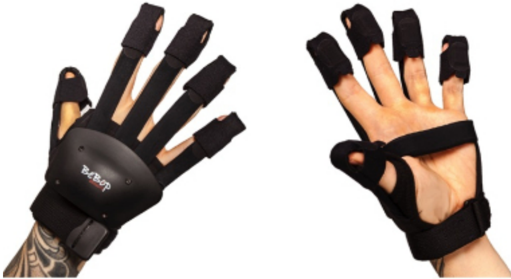
Figure 3.3.1: BeBop gloves ( https://bebopsensors.com/ ) with six sensors on five fingertips and palm. Picture originally from Courtesy BeBop Sensors Thomas PR.
