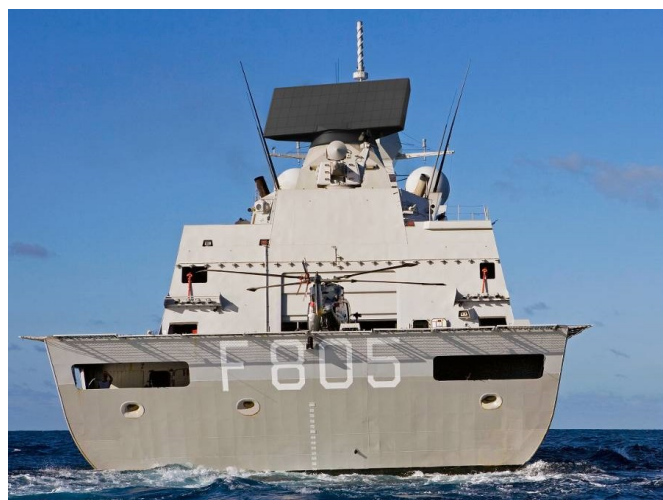
The Thales Smart-L radar on top of a defence frigate.
