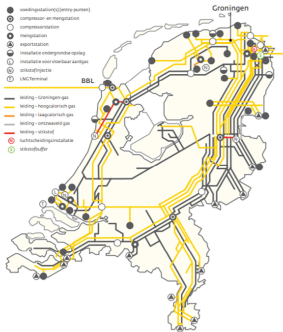
Figure 1 Schematic Main Gas Network Netherlands (Gasunie, 2020)
