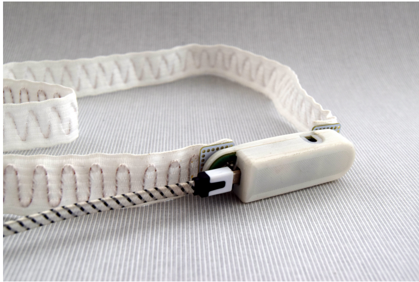
Figure 1.2: The current version of the Breathline with RIP belt and USB cable connected
