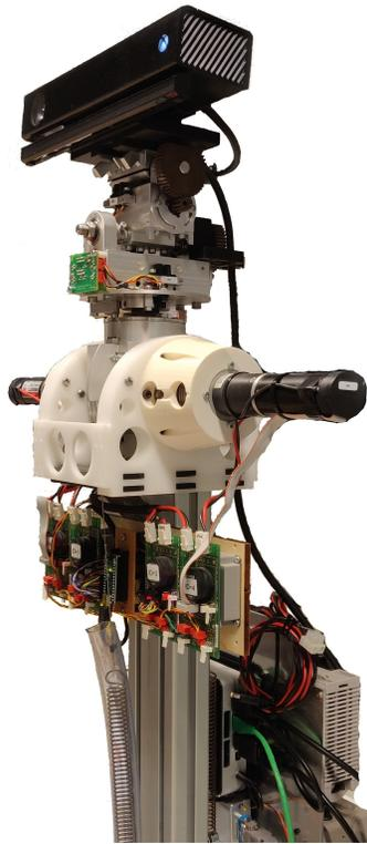
Fig. 2: The Twente humanoid head platform used to accommodate for the movement of the Kinect 2.
