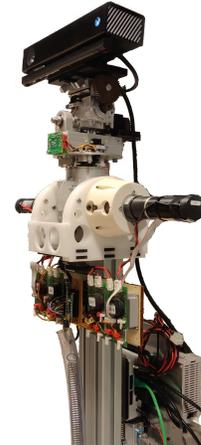
Fig. 2: The Twente humanoid head platform: a moveable platform for the Kinect 2 sensor.
