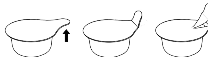
Figure 16. Built-in opening mechanism of the current coffee creamer portion packaging.
