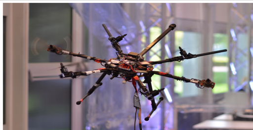
Figure 1.2 Fully-actuated hexarotor hovering at a non-zero pitch and roll angle [Rashad et al., 2019a]
