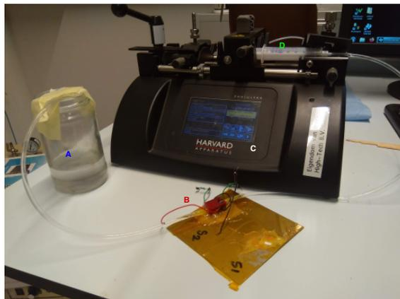
**Figure 5.4:** Syringe pump setup
