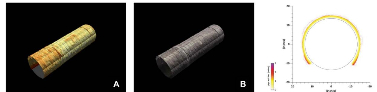
Figure 0-16: Example of the 3D pipe model with LIDAR data projection (left, A); 3D CCTV image as a comparison (middle, B); Right: summarized inner pipe-wall geometry based on LIDAR data, the black line represents the original pipe diameter, source from (Ekes, et al., 2012).
