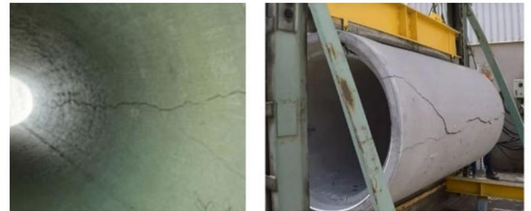
Figure 0-4: inner pipe cracks (left) and outer pipe cracks (right).
