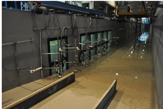
Figure 3.2: Wave flume experiment set-up with the attached PPT and AWG on the poles (The picture is retrieved from Sara Dionisio Antonia who participated in the wave flume experiments).
