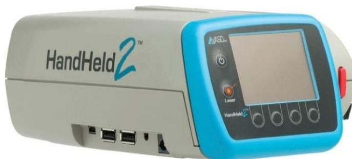
Figure 9 ASD FieldSpec handheld 2
