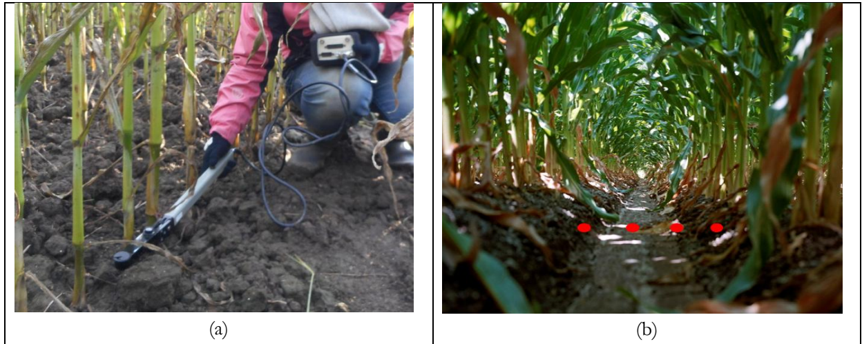
Figure 4: Photograph of the LAI measurement procedure; a) shows example of an independent LAI measurement, b) outlines the various measurement positions (photographs taken on 2016/11/11)
