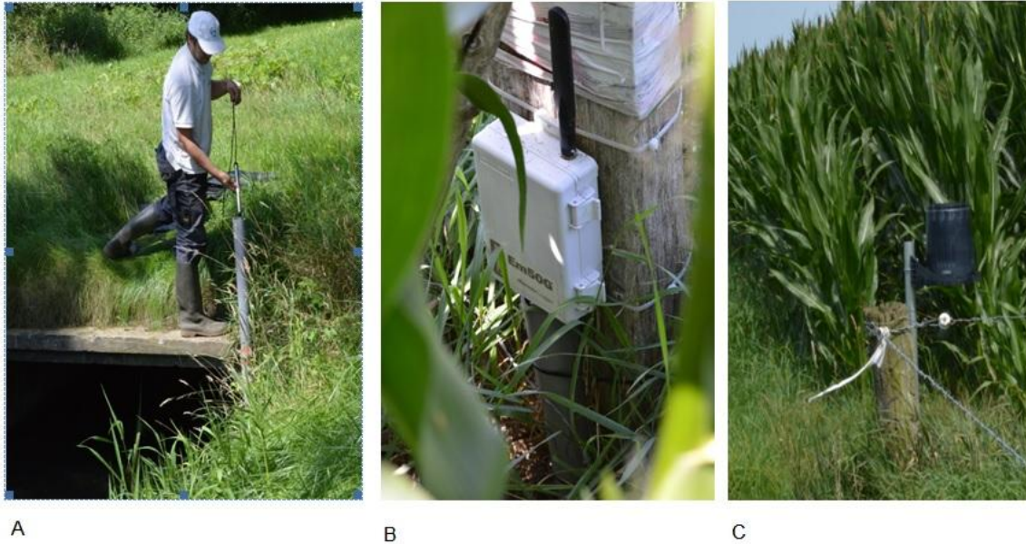
Figure 7: ITC stations within the Voltherbeek (A) water level station (B) soil moisture station (C) rainfall gauging station
