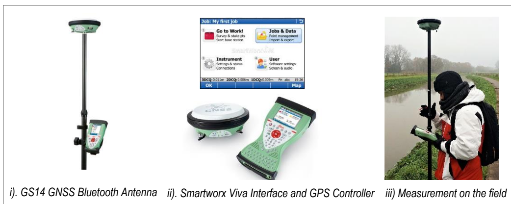
Figure 2. 10. RTK GPS Instrument, Smartworx Viva Interface, and Field Measurement
