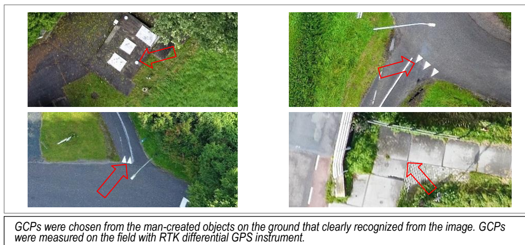
Figure 2. 4. Ground Control Points (GCP) features
