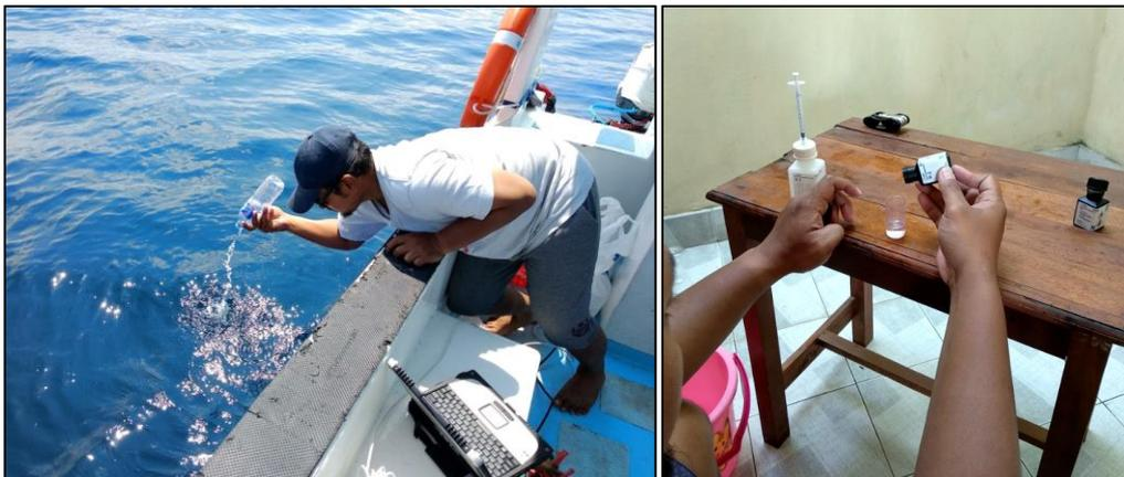
Figure 9. Seawater sampling (left) and Total Alkalinity measurement (right).
