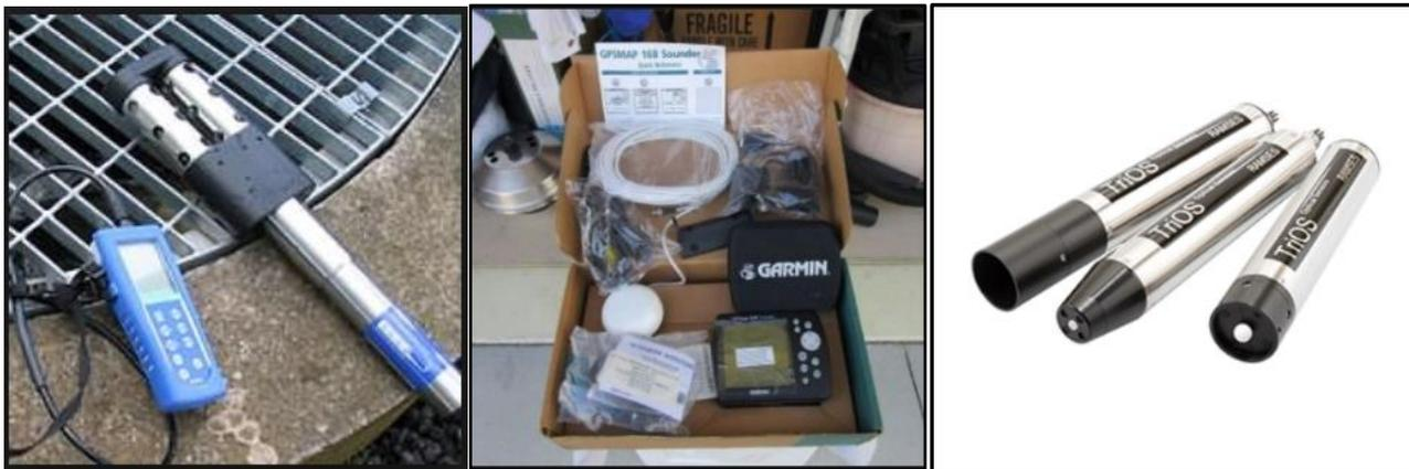
Figure 10. Instrument used for field measurement in this research are TOA-DKK WQC 24 (left), Garmin GPSMAP sounder (middle) and Trios Ramses (Right).
