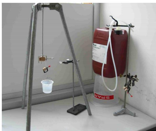
Figure 2-8. Device designed to measure tensile strength (Pohl, 2010).
