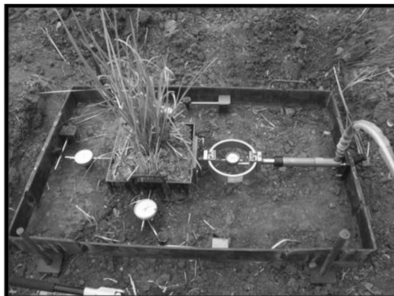
Figure 2-4. In situ direct shear test (Teerawattanasuk et al., 2014).
