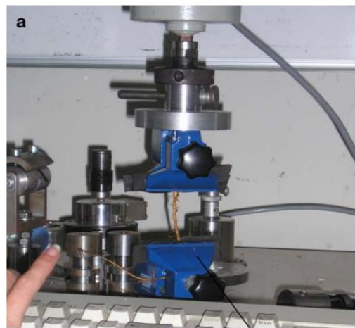
Figure 2-7. UTS apparatus to perform root tensile strength tests (De Baets et al., 2008).
