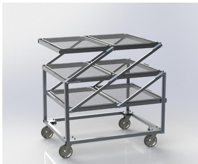
Figure 1: Final cantilever rack design.
