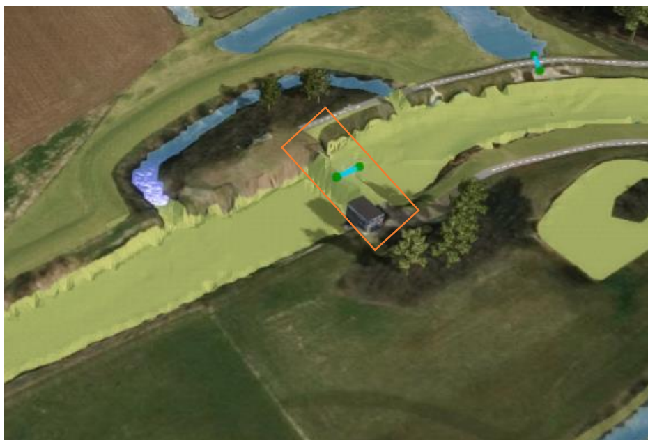
B3-4. To prevent a weir from leaking water under and past the weir, the elevation at the weir location is increased. The orange rectangle indicates the elevated area and the blue line indicates the weir with entry/exit points. The area is increased to a surface level of 12 m+NAP at De Haandrik and 9.5 m+NAP at Hardenberg.
