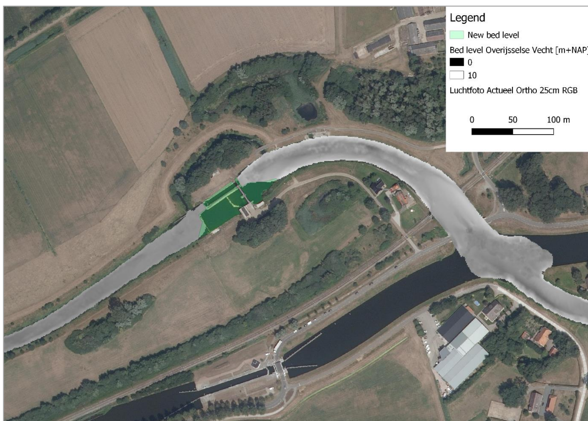
B2. A close-up of the measured bathymetry at weir De Haandrik and the crossing with the Almelo Kanaal. In this figure is visible that it was not possible to measure the entire trajectory between De Haandrik and Hardenberg. Manual additions to the bed level were needed to fill the unmeasured area at e.g. weir De Haandrik, (green shape).
