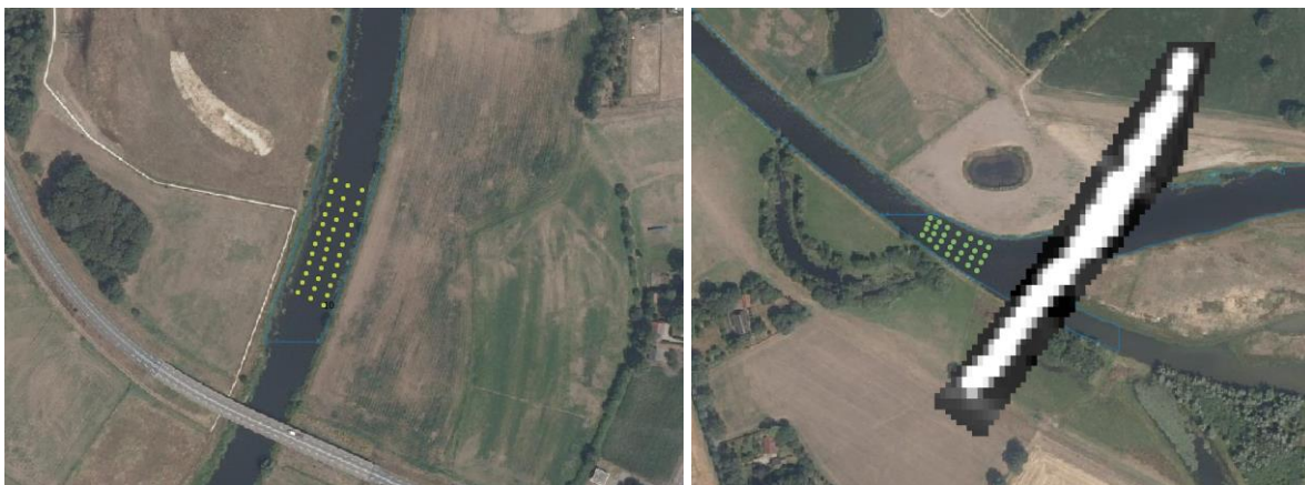
Figure 13: 33 inlets are used to define the lower boundary condition (left figure). Each row represents a water level (in descending order from north to south) over which the corresponding discharge is defined over 3 inlets in width. The middle inlet contributes to 60% and outer inlets contribute to 20% of the related discharge. The right figure presents the 28 inlets used as an upper boundary condition where the discharge is equally distributed over the length and width of the channel. The greyscale in the right figure presents the dam as a rasterized area where the height is increased to 20 m.
