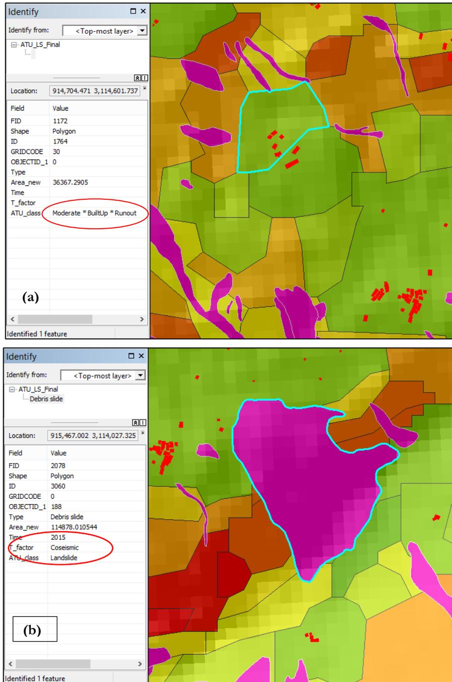
Figure 4.16: Attribute information of selected automated terrain unit (a) other than landslide unit and (b) landslide unit
