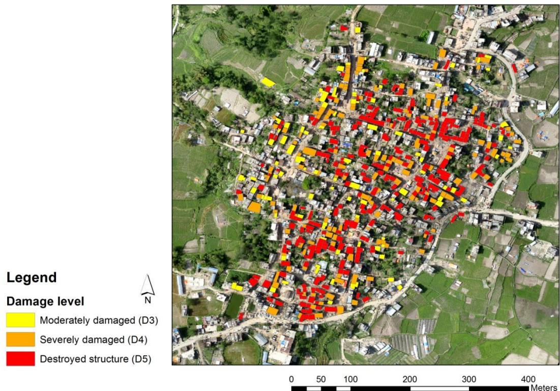
Figure 12 Damage map of Sankhu area. Map is created by analysing the orthomosaic that was created from ICIMOD images (original map)
