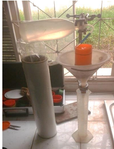
Figure 2.4 Saturated hydraulic conductivity apparatus
