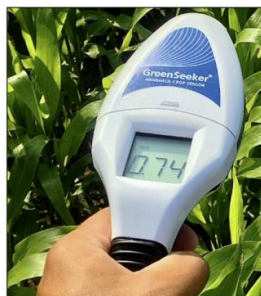
Figure 2.5 Equipment for field NDVI measurement
