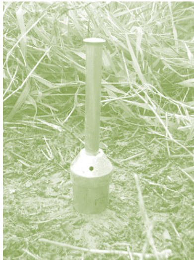
Figure 2.3 Undisturbed soil sampling in the field
