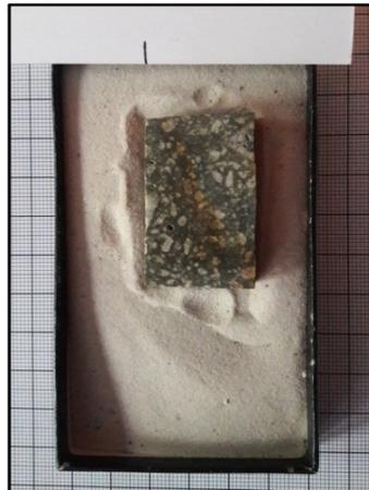
Figure 4. Sample block placed in the box for the measurement
