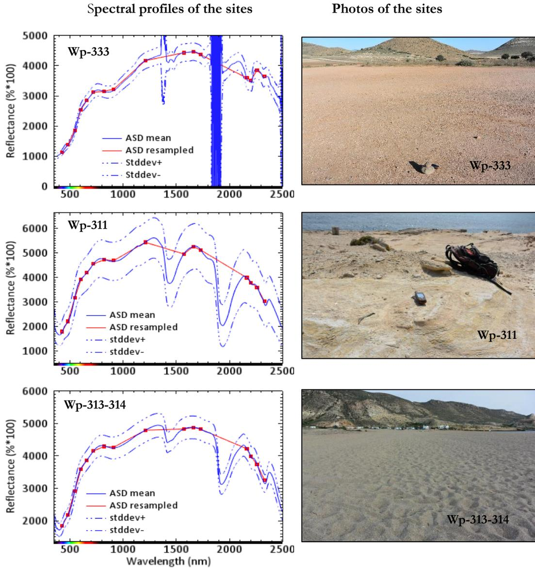
Figure 4. Spectra of the reference sites collected by ITC staff in Rodalquilar, September 2017: measured ASD field spectra (blue) and resampled to WV-3 spectra (red). Photos of the sites are provided on the right. The locations of these sites are shown in Figure 3.
