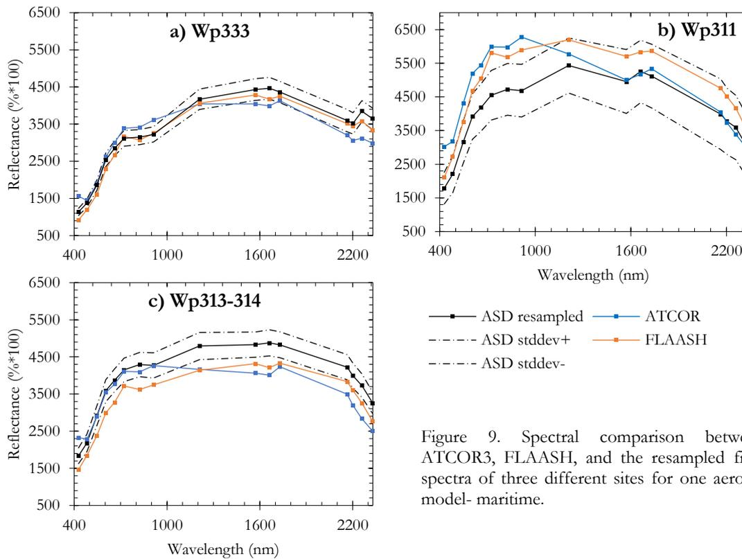
Figure 9. Spectral comparison between ATCOR3, FLAASH, and the resampled field spectra of three different sites for one aerosol model- maritime.
