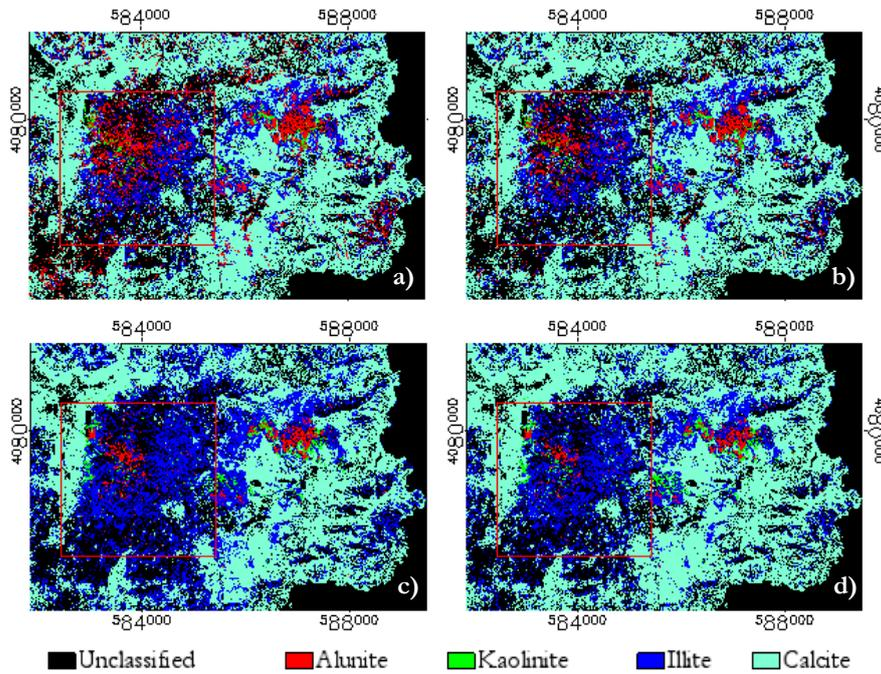
Figure 18. Mineral maps produced from SAM classification method with 0.1rad threshold. a) May-AComp, b) May-FLAASH, c) Sept-AComp, d) Sept-FLAASH.
