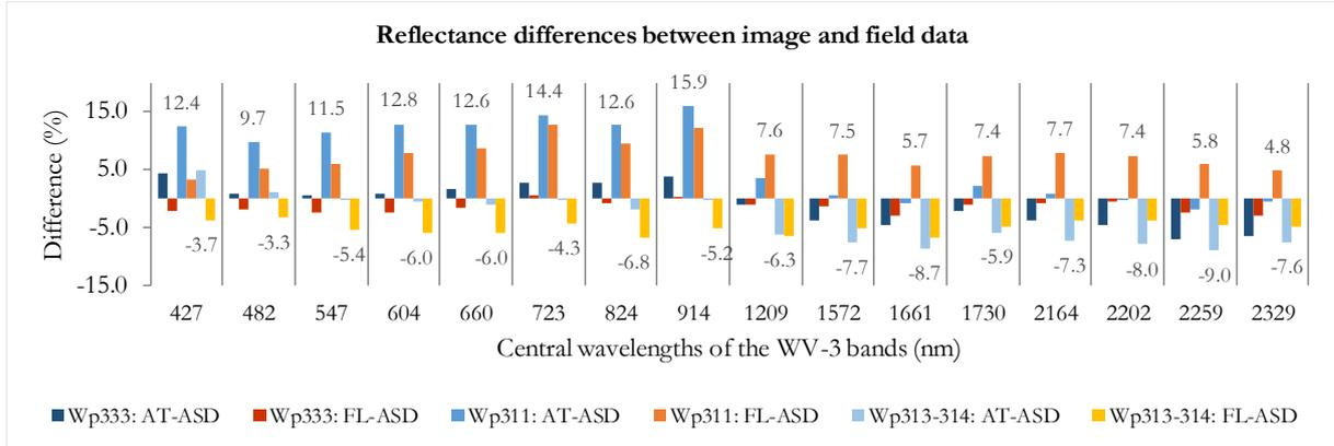
Figure 10. Differences of the surface reflectance estimated by ATCOR3 (AT) and FLAASH (FL) and measured in the field (ASD- resampled to WV-3 bands) of three reference sites. Positive values show overestimation and negative values show underestimation of the reflectance compared to the field data. The highest positive and negative values are labelled.
