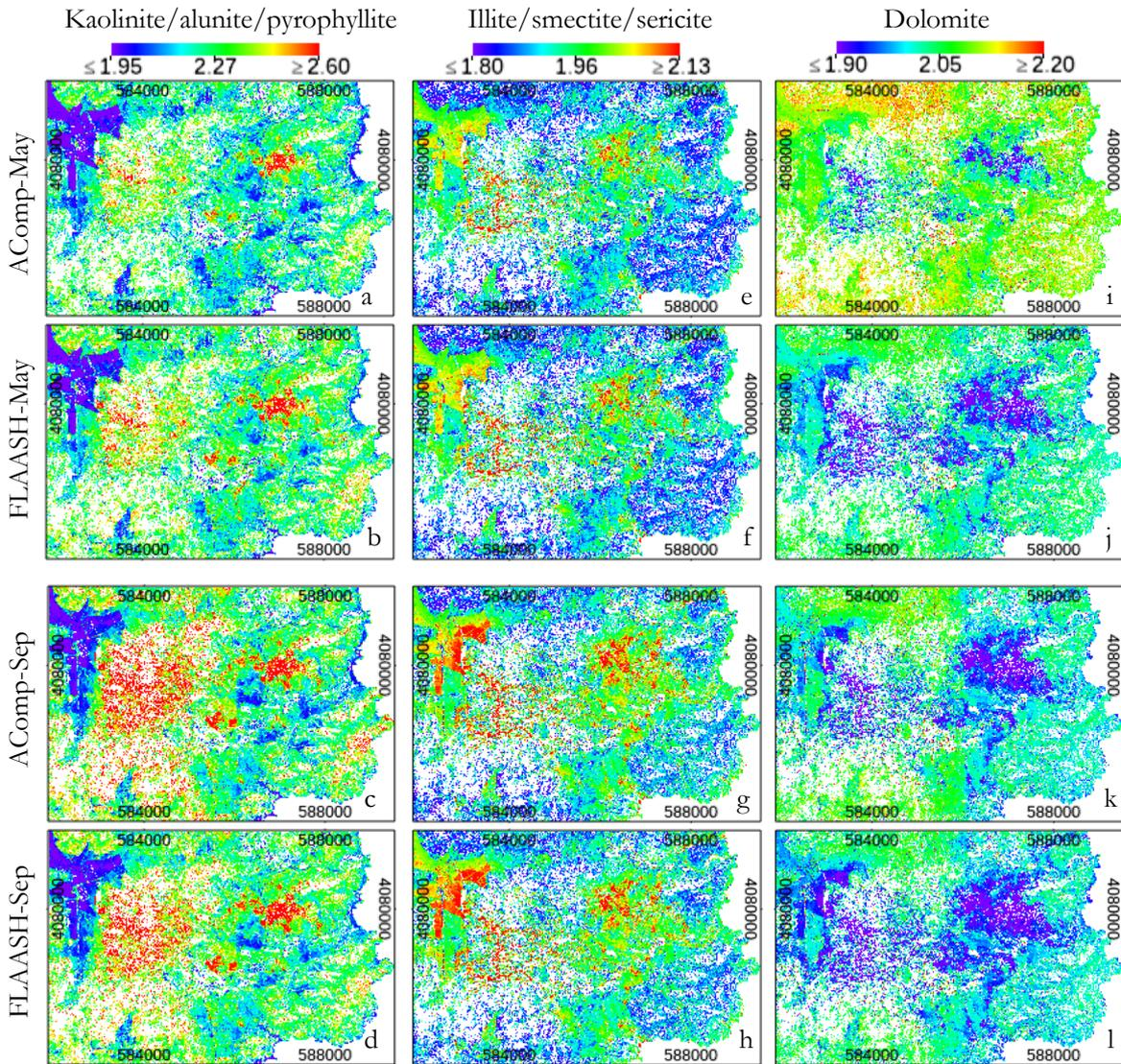
Figure 16. Band ratios defined by Rowan (USGS) for ASTER bands. Kaolinite/alunite/pyrophyllite, illite/smectite/sericite and dolomite ratios produced from AComp and FLAASH corrected WV-3 images. The top two rows show May images and the bottom two rows show September images.
