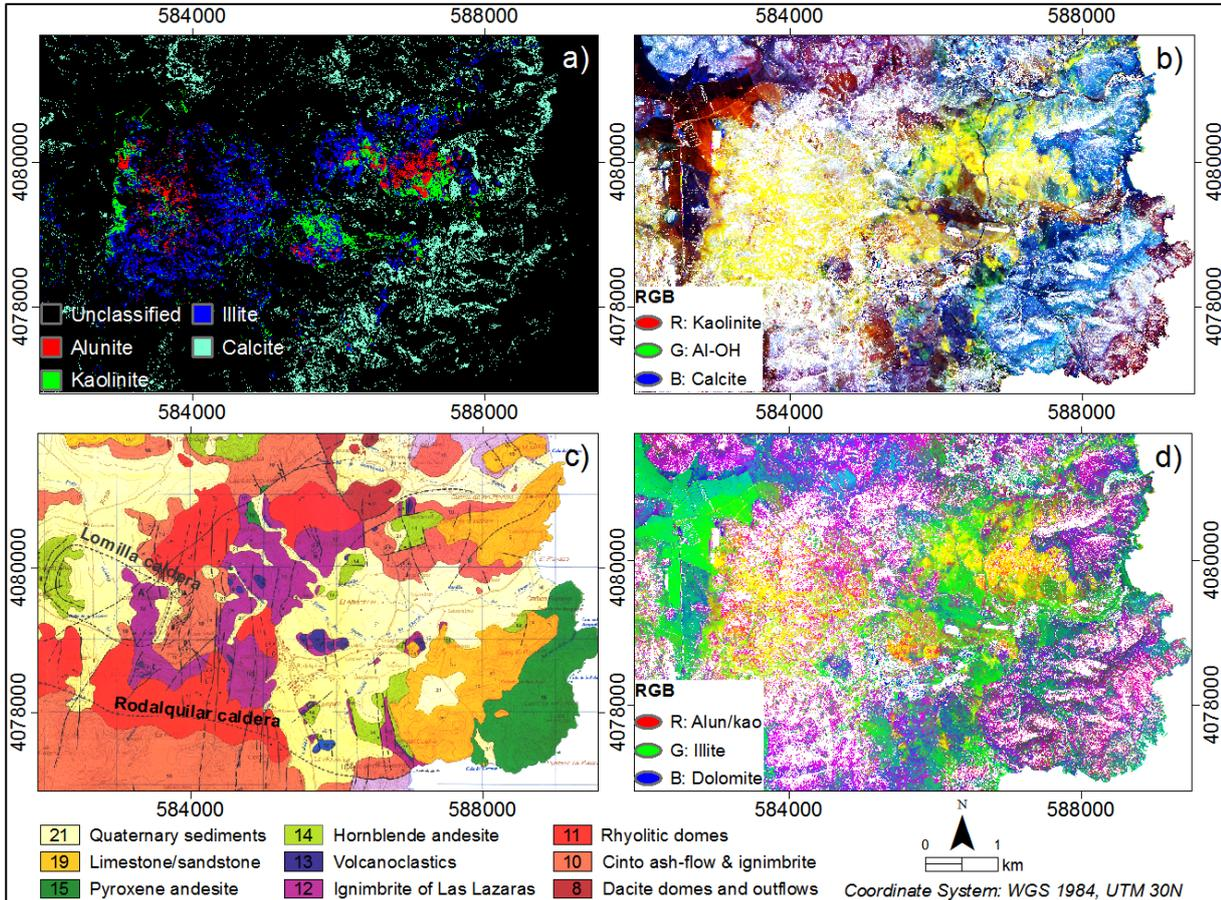
Figure 25. Comparison of geological map with the mineral maps produced from the band ratios and the classification using SAM. a) SAM classified image with 10% threshold, b) A colour composite image made of Sun's mineral indices, c) Arribas' geological map, and d) A colour composite image made of Rowan's band ratios.
