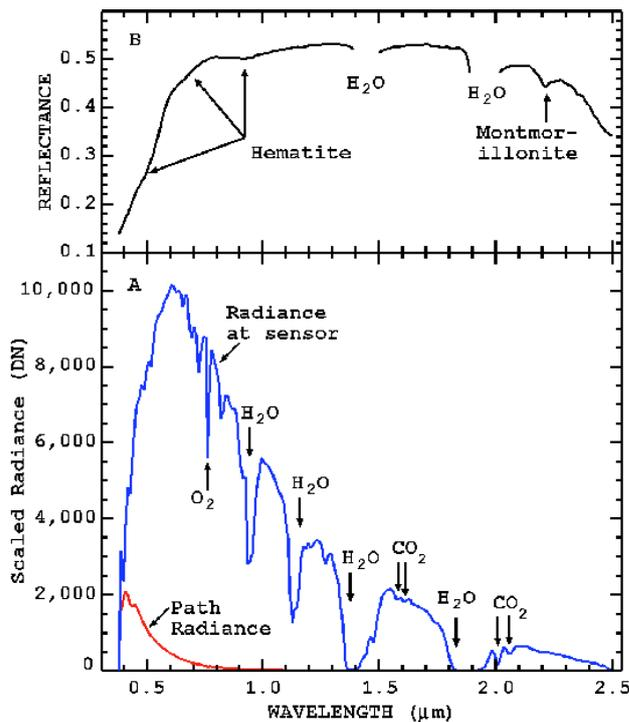
Figure 5. An example of reflectance and radiance spectra. A- radiance spectrum of non-vegetated area and B- the surface reflectance spectrum after atmospheric correction (Clark et al., 2002).
