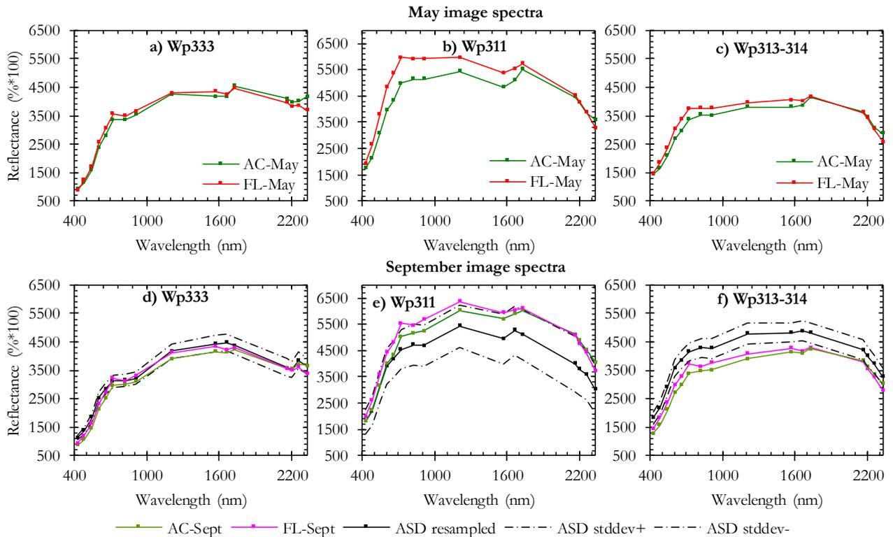
Figure 12. Spectral comparison of AComp (AC) and FLAASH (FL) corrected WV-3 images of May and September acquisitions for each reference site. September image spectra compared with resampled field spectra, yet for May image, in-situ data has not been collected.
