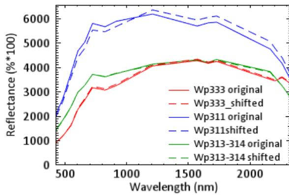
Figure 23. Spectral profile of the reference sites before and after correcting geolocation difference.
