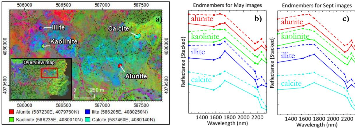
Figure 17. a) Location map of ROIs used for endmembers and their coordinates of the centre point overlaid on DS image. b) Endmember spectra for May images, c) Endmember spectra for September images. Solid lines are AComp image spectra and dashed- FLAASH image spectra.
