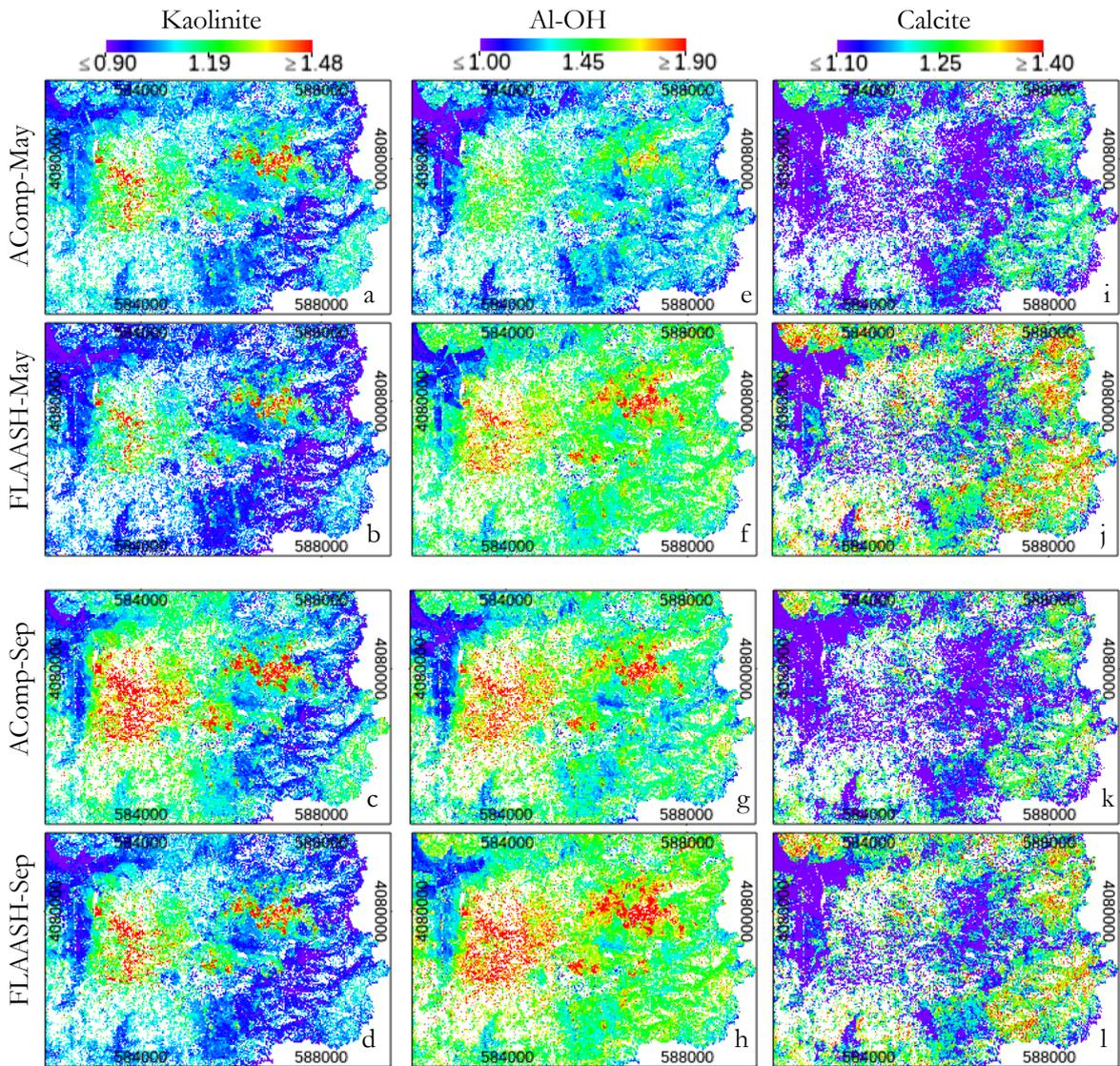
Figure 14. Kaolinite, Al-OH and calcite mineral indices maps produced from AComp and FLAASH corrected WV-3 images. The top two rows show May images and the bottom two rows show September images.
