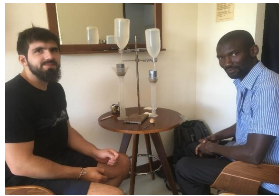
Figure 2-13: Assessment of saturated hydraulic conductivity with makeshift permeameter
