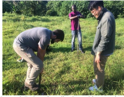
Figure 2-7: Sample collection with a spade and assessment of soil depth with a soil auger
