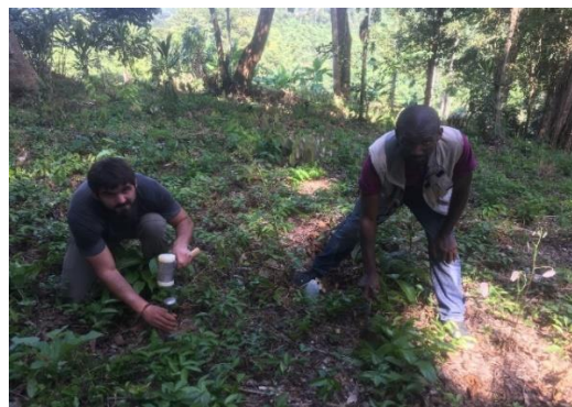
Figure 2-9: Sample collection with sample rings and shear strength assessment of level land
