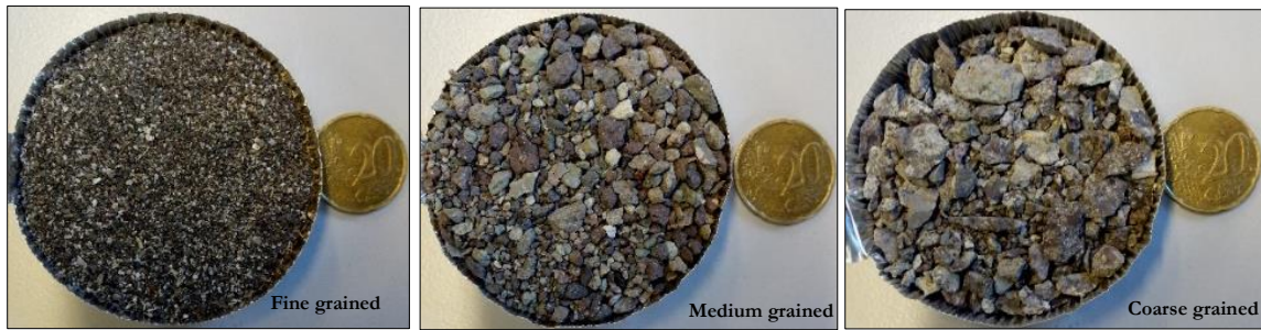
Figure 3-2: Images of various grain sizes of drill cuttings from OW-917.
