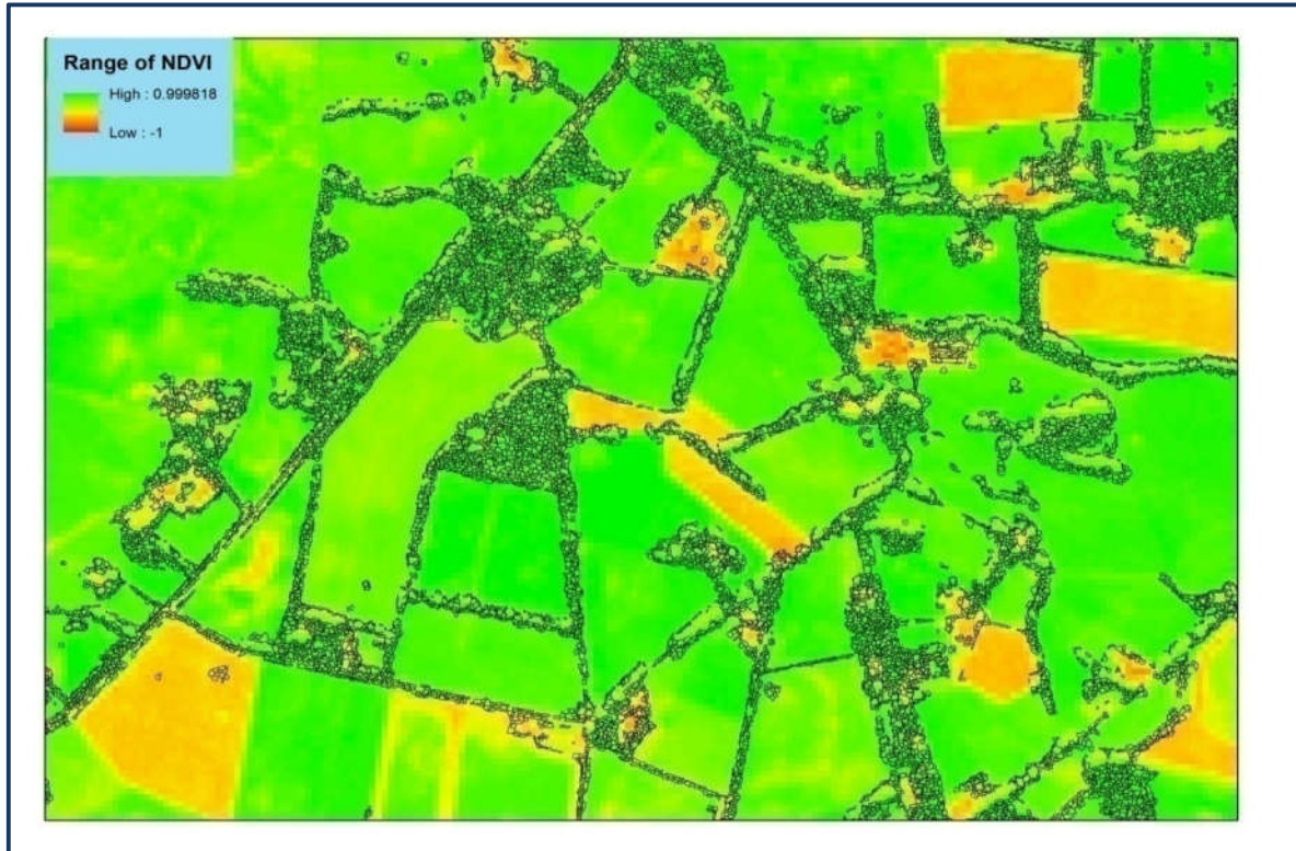
Figure 2-8: Overlay of tree crown from VHR image (Pleiades) with NDVI of Sentinel-2 data
