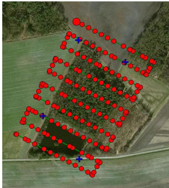
Figure 29: Flight plan (green line and red image taking positions) and GCPs (blue crosses) for flight area 3
