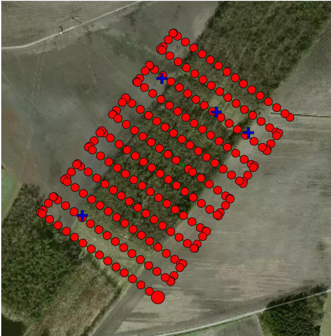
Figure 6: Recorded flight plan for flight area 4. Red dots indicate the position of the UAV where an image was taken (measured by on-board GPS). The big red dot in the lower right corner indicates first picture taken from the UAV. The blue crosses mark the position of ground control points.
