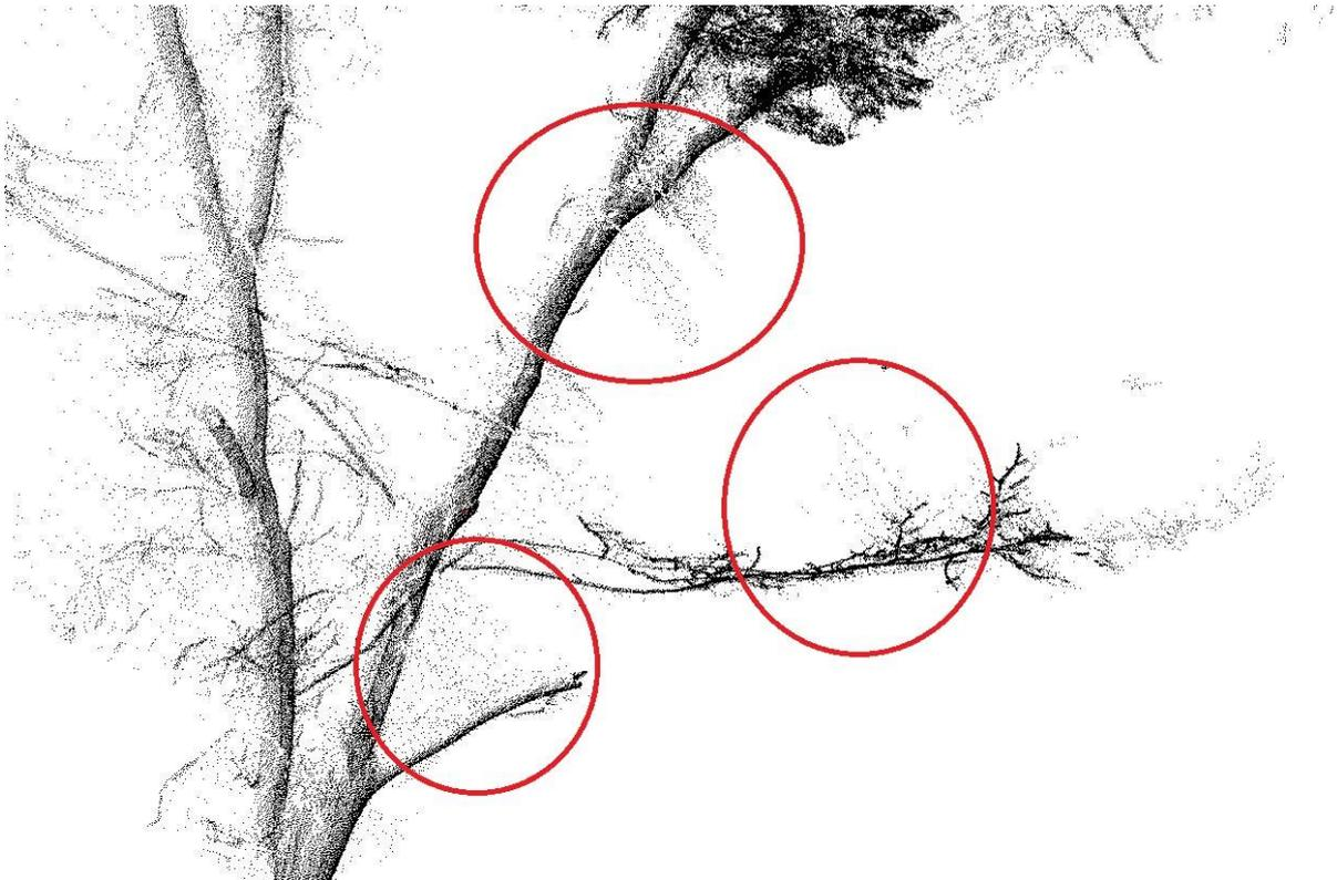
Figure 21: The occurrence of “shadows” of points behind objects (see red circles) add to general complexity of structures and make the recognition of interconnected and separated objects as well as the recognition of finer structures difficult.
