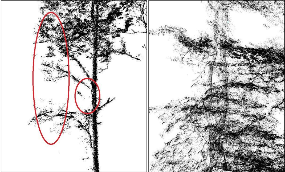
Figure 20: left: Occlusion of structures/objects (see red circles) make recognition of connected structures (e.g. branches) difficult. Right: Intertwined tree stems that cannot effectively be separated and create errors especially when measuring DBH.
