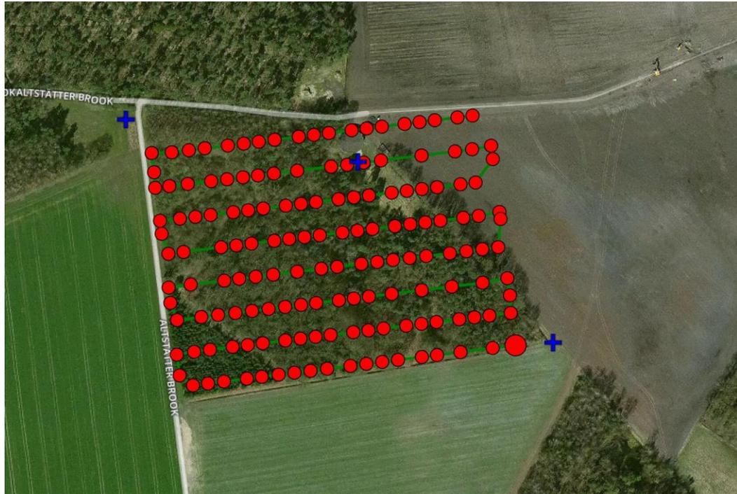
Figure 28: Flight plan (green line and red image taking positions) and GCPs (blue crosses) for UAV flight area 1
