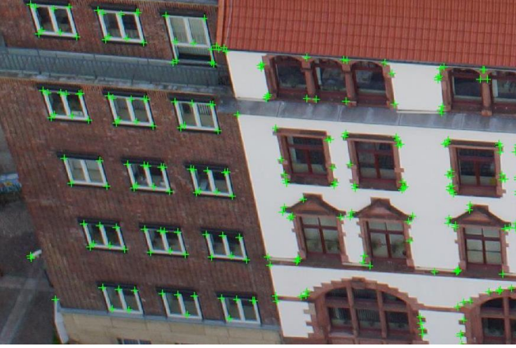
Figure 2.2: Harris corners detected marked with green crosses.
