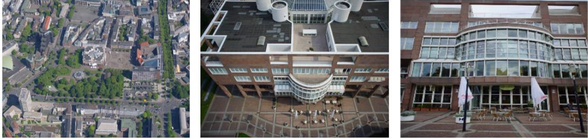
Figure 1.1: Left: Airborne oblique image. Centre: oblique UAV image. Right: Terrestrial image.
