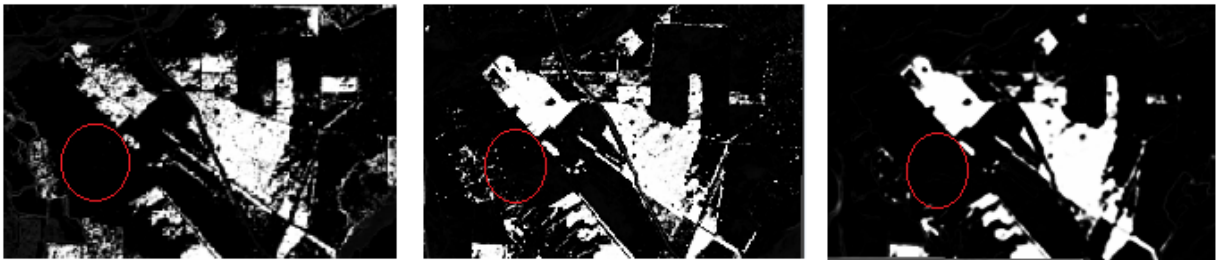
Figure 6.12: Example of fuzzy local spatial information classifier in removing isolated pixels. (a) Reference fraction image for eucalyptus class (b) FCM classifier output fraction image with isolated pixels (c) FLICM classifier output fraction image where isolated pixels are handled
