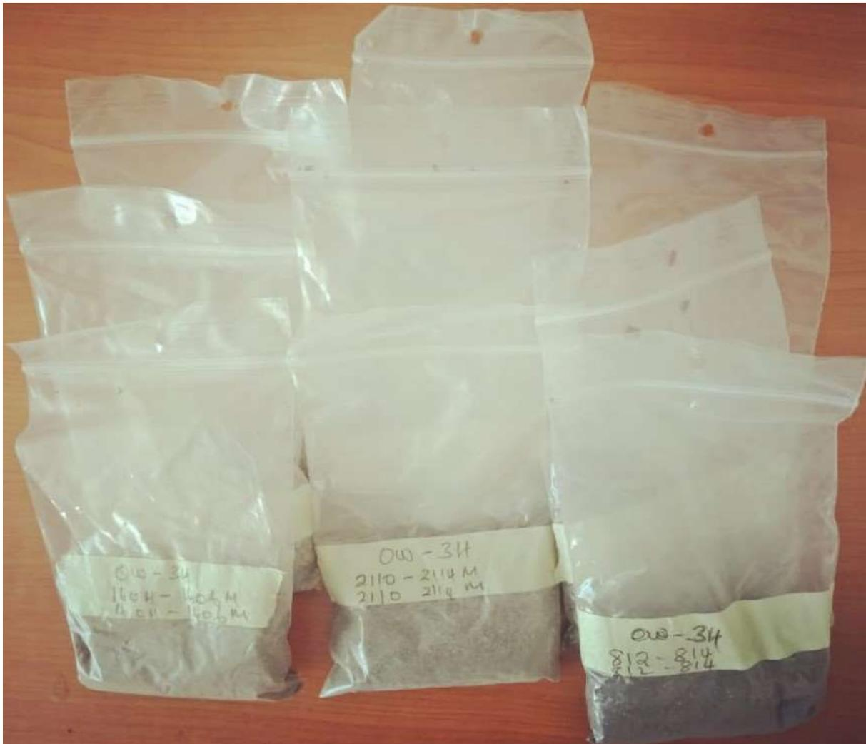
Figure 5: Image showing some of the collected geothermal drill cuttings. Sample identification including well ID and depth of sampling
