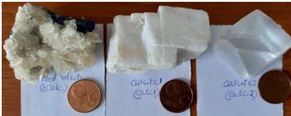
Figure 4: Calcite sample varieties used in the study. From left to right; Bcalc, Calc1, and Calc2 respectively. Note that the triangular plane on Calc2 is not a facet/cleaved plane but a cut surface.
