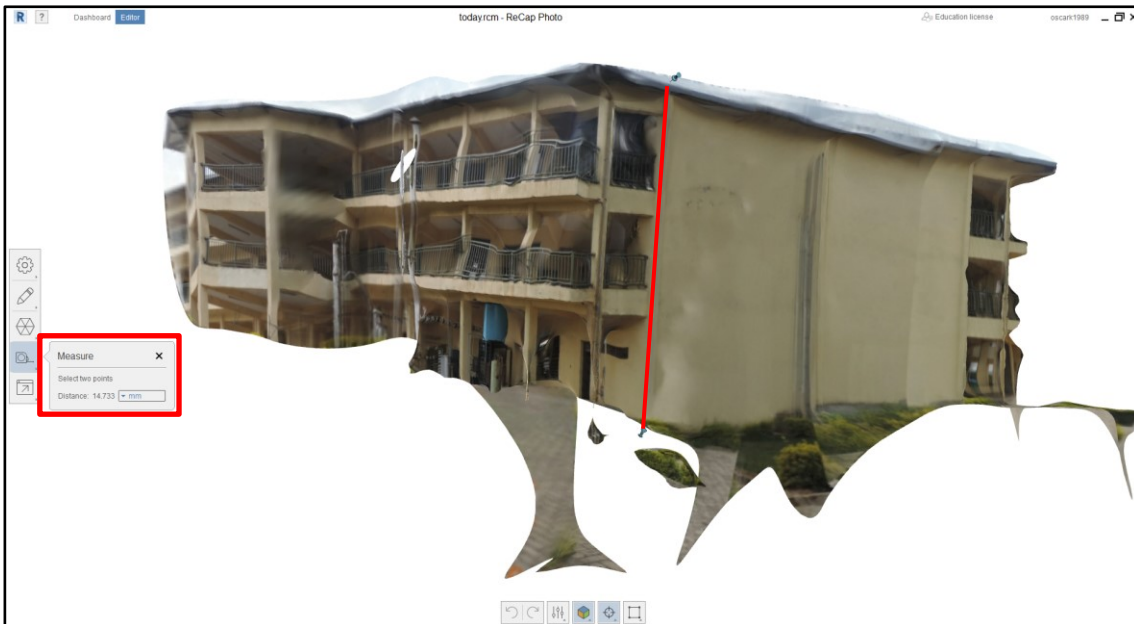
Figure 4-8: Generated 3D model from terrestrial images showing that from the model the height of the building can be measured
