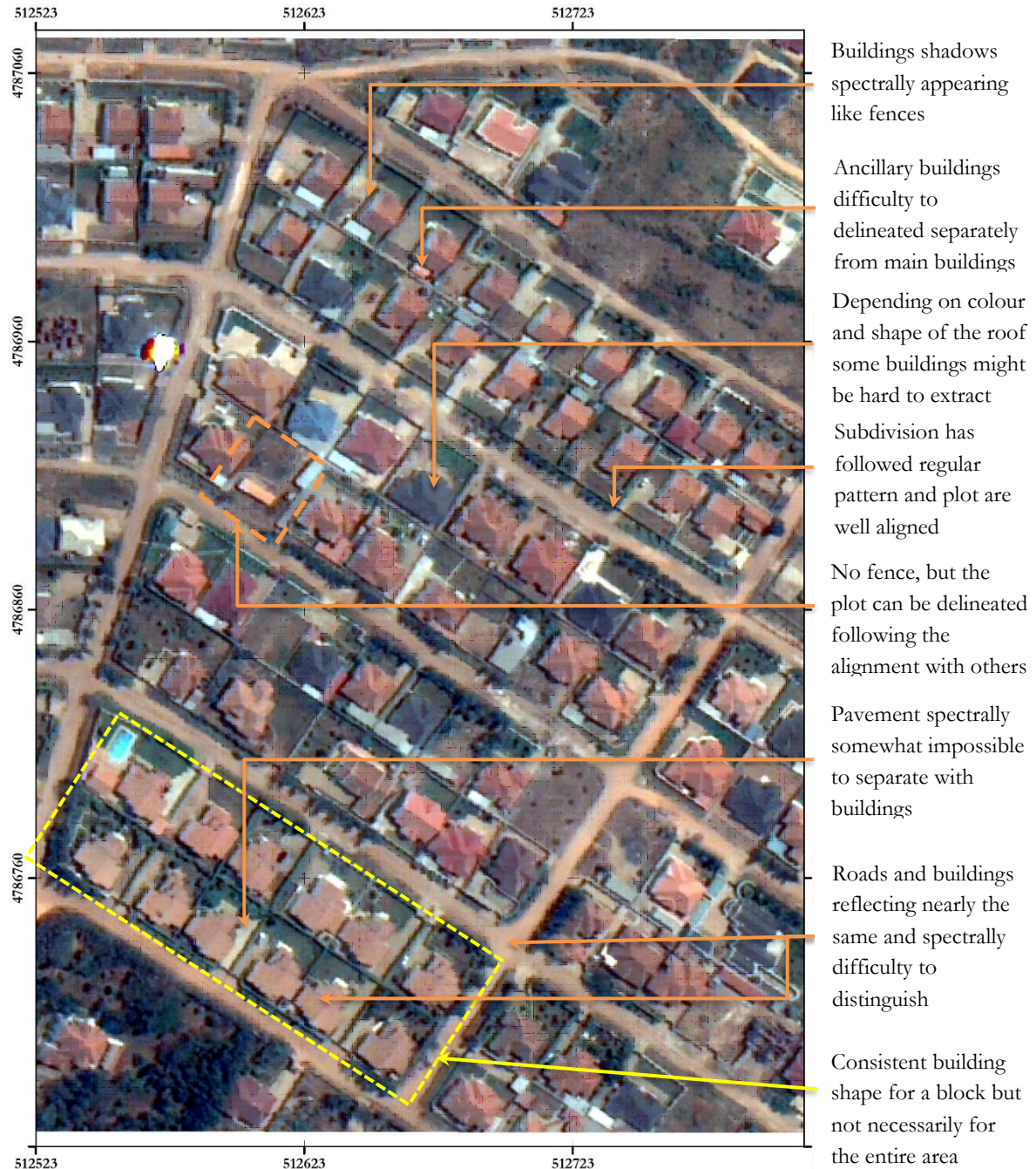
Figure 14: Appearance of building roof and fences on image
