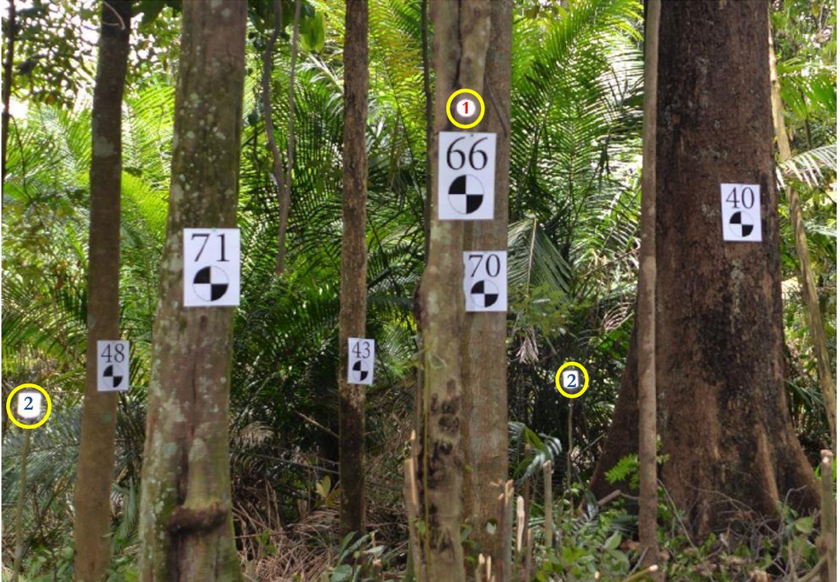
Figure 3.5: circular retroreflectors (1) and cylindrical retroreflectors (2)
