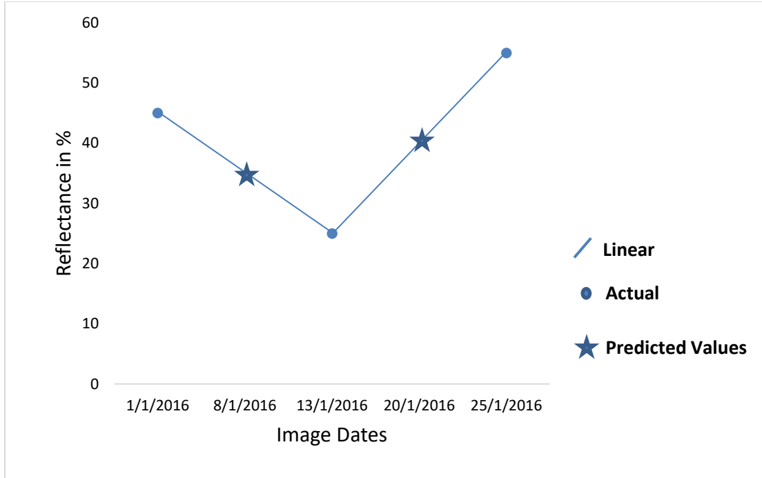
Figure 2-9: Linear interpolation function
