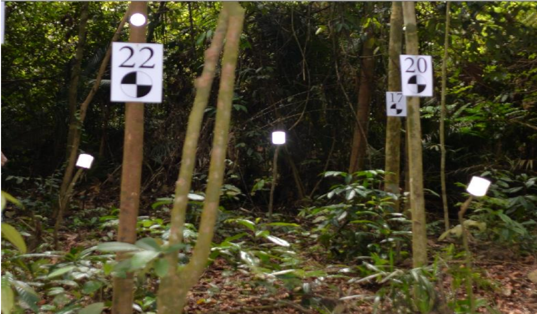
Figure 3.6: Distribution of retro-reflectors inside the sample plot
