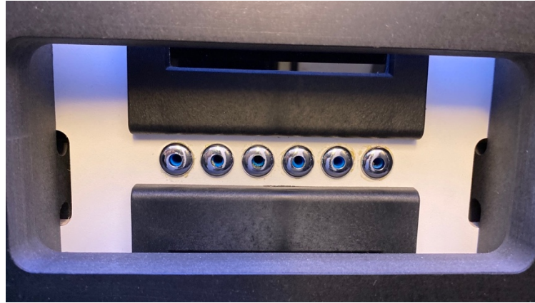
Figure 9-14: The scent dispenser has six holes for six fragrances.
