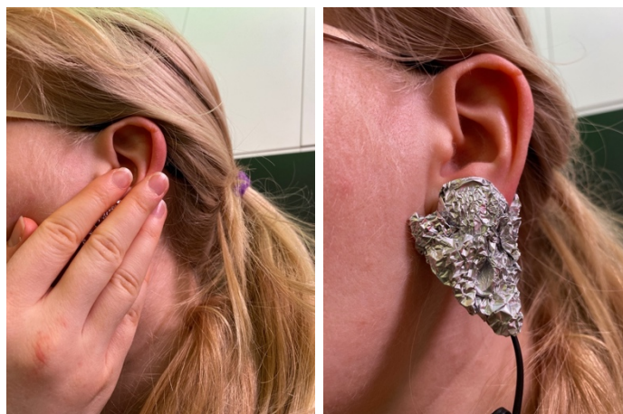
Figure 9-25: Blocking out the infrared light from the heat panels using a hand and aluminium wrap was not effective.
