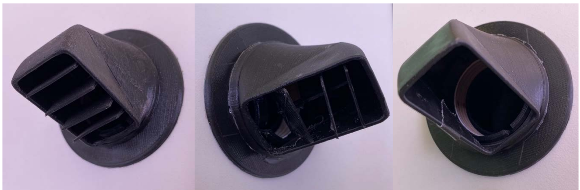
Figure 9-10: Ventilator caps. Left: with intact grilles. Middle: with broken grilles. Right: with no grilles.
