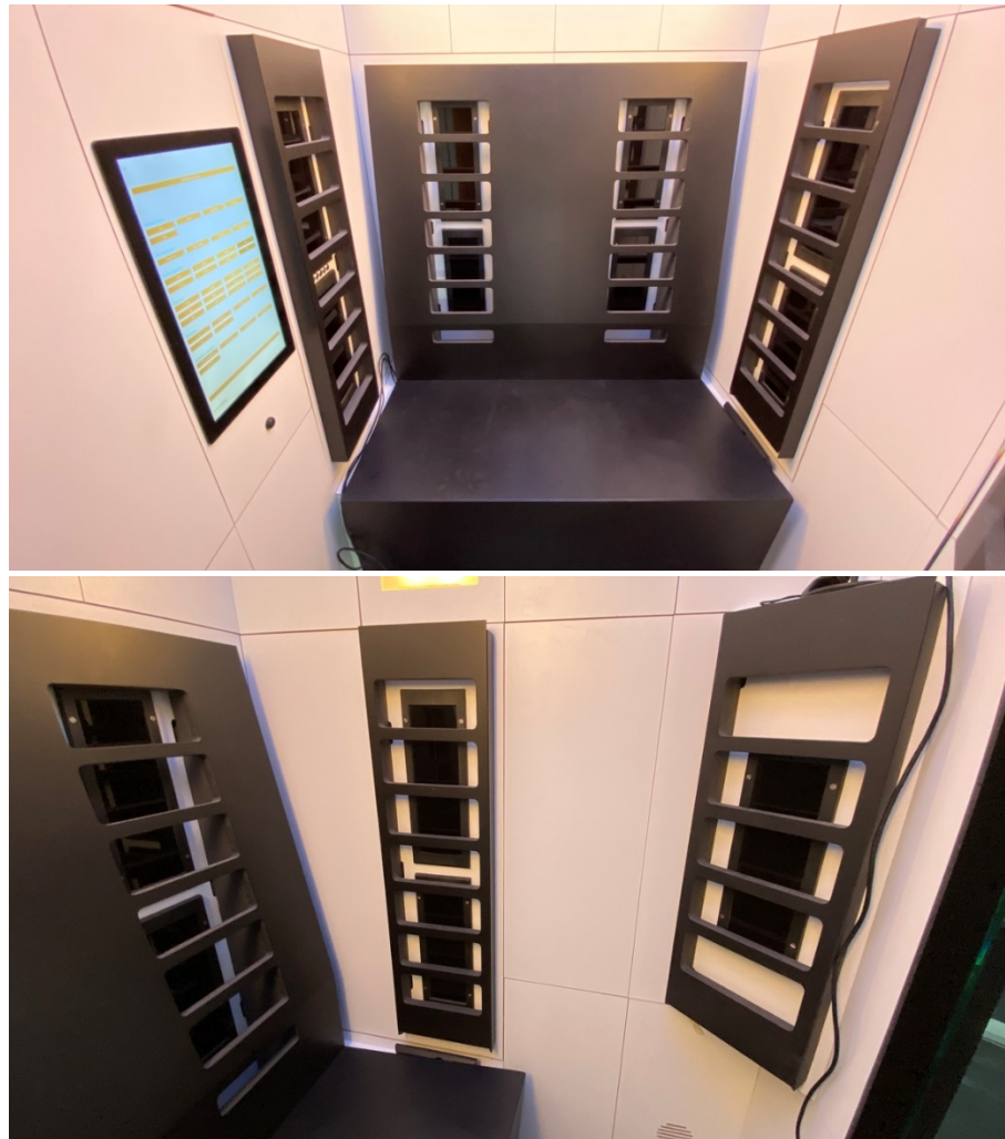
Figure 9-11: Infrared heating panels are covered by wooden frames to avoid the user getting burnt.
