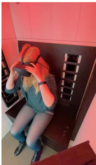
Figure 9-18: Light panels correspond to the colour scheme of the virtual reality content and are turned on even when the virtual reality headset is used.
