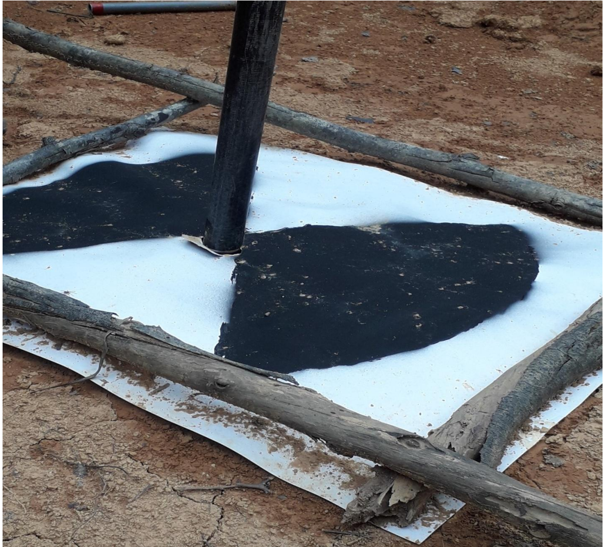
Figure 11: 45 cm X 60 cm Marker and plastic tube inserted at centre.
